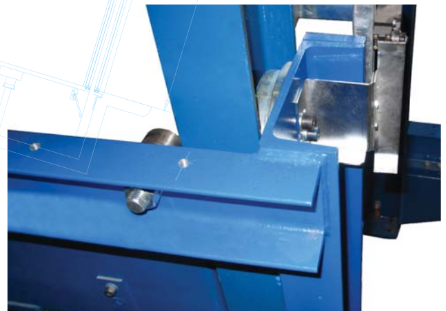
Figure 6. Lateral Guiding, 4 bearings per frame.
