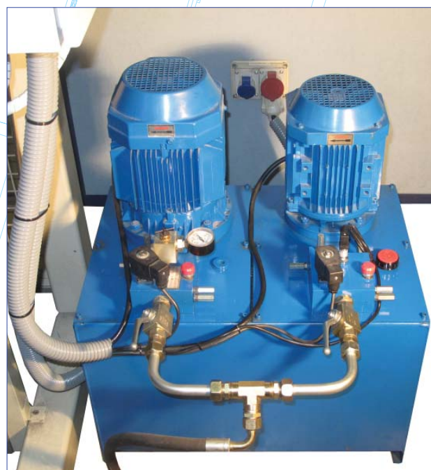
Figure 17. Central Hydraulic Unit.
